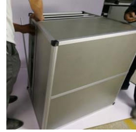
12: Insert the three round tubes into the holes, and use one bar to fix with the back wal, then fix the other side panel
